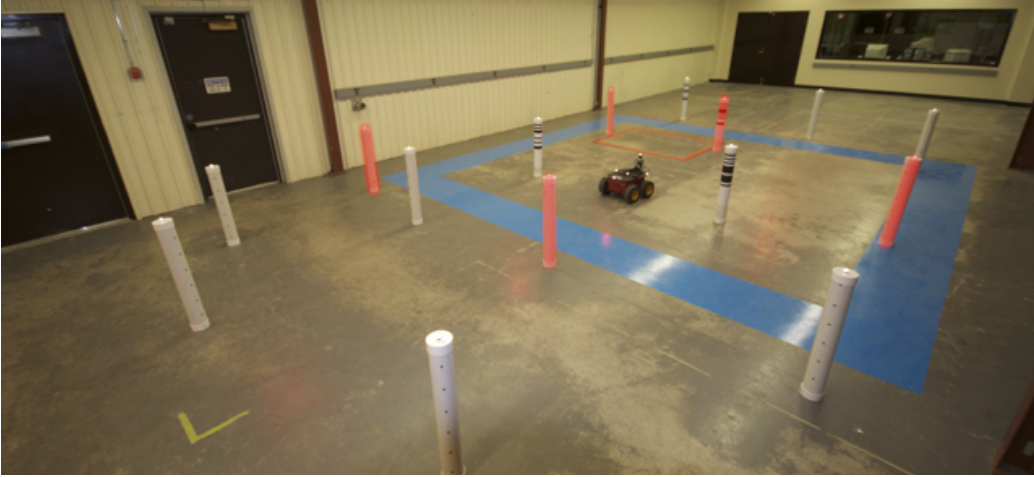
Figure 6.7: Setup for Experiment 1. A wheeled robot drives around 17 cylindrical landmarks (2 are not visible in this photo) in an indoor environment. It logs wheel odometry and measures the range to its surrounding landmarks using a laser rangefinder. The landmarks for testing are highlighted in red.
